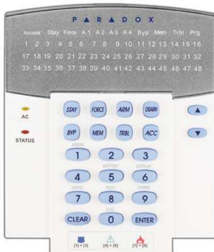
Figure 2: DGP2-648BL LED Keypad Overview
