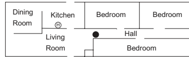
Smoke detectors should be located between the sleeping area and the rest of the family living unit.
